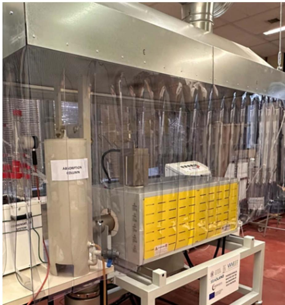
SEACURE is validating the production of **bio-based fertilisers (BBFs)** derived from biosolid wastes in wastewater treatment plants (WWTPs), transforming them into comprehensive resource recovery facilities. Building on knowledge from the H2020 SEA2LAND and PROMISCES projects, thermochemical processes are applied under oxygen-limited conditions to recover nutrients from sewage sludge and organic wastes, concentrating nutrients in biochar while removing organic contaminants and toxins.
